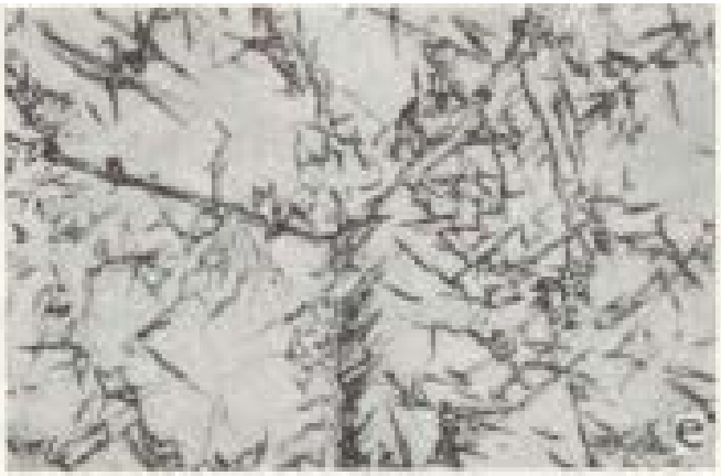
FIG. 62. Widmanstätten structures. (a) Brass, cast (for phase diagram, see Fig. 392, p. 510). \alpha (light) precipitated in \beta (dark), etched in alcoholic ferric chloride. \times 30 . (b) Similar material but containing less \alpha and showing clearly the varying orientation of the \beta grains. \times 50 . (c) \alpha - \beta brass, but showing reversal of etching by ammonium persulphate. \times 50 . (d) Brass, cast: \gamma -phase precipitated in \beta . \times 50 . (e) Copper-4 per cent beryllium (phase diagram, Fig. 384, p. 503). Quenched from molten condition in water: incipient or arrested precipitation of \alpha in metastable \beta . \times 700 .
