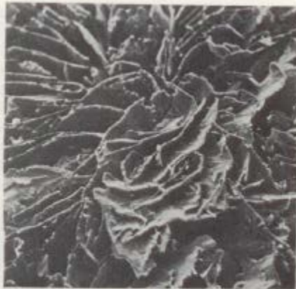
Scanning electron micrograph of flake graphite in cast iron, showing the gross distortion and the interconnected nature of the graphite (x 5000) (Courtesy of M. G. Day, B.C.I.R.A.)
