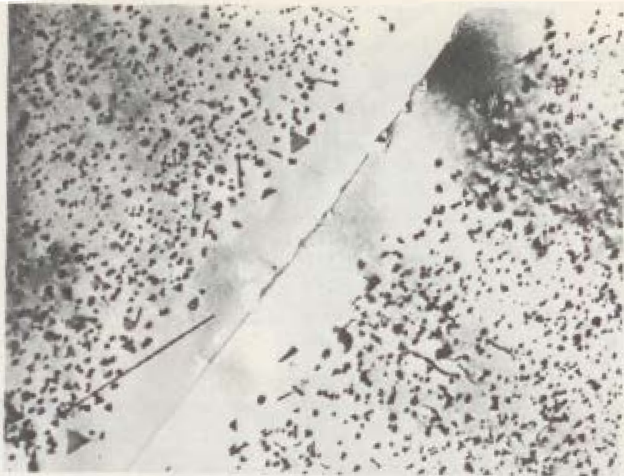
Figure 6.13 Precipitate free zone around a grain boundary in an Al-Ge alloy (x 20 000) (Courtesy of G. W. Lorimer 6 )
