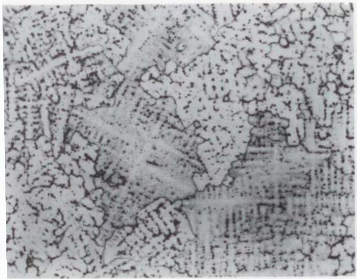
9/30 brass etched in alcoholic ferric chloride, showing cored grains, and interdendritic constituents. 100x.
