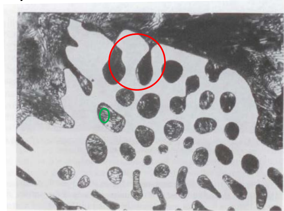
Fig. 121. Some pearlite in the ledeburite is resolved as well. 1000x.
