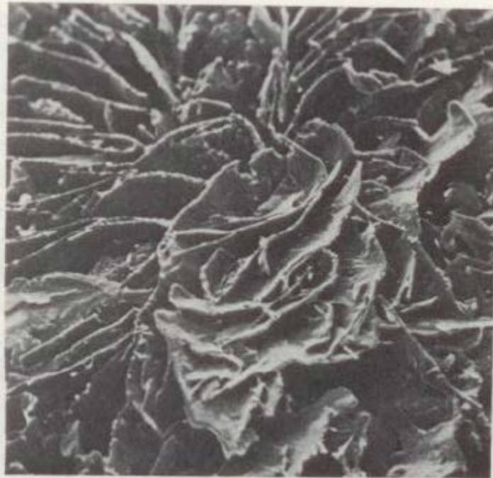
Figure 4.66 Scanning electron micrograph of flake graphite in cast iron, showing the gross distortion and the interconnected nature of the graphite (x 5000) (Courtesy of M. G. Day, B.C.I.R.A.)
