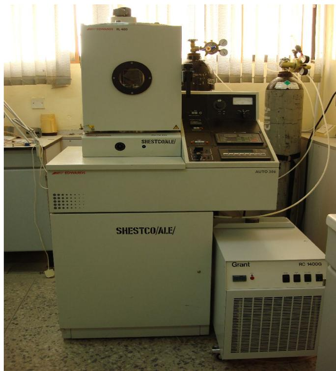
**Fig. 2.4: Edwards Auto 306 Thermal Vacuum Evaporator**
