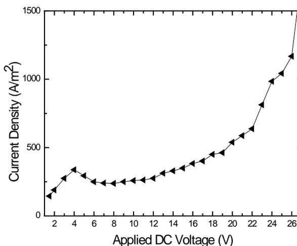
**Figure 4.** Electro-polishing current density-voltage curve for perchloric acid in alcoholic electrolyte for aluminum sample area 0.0008 m<sup>2</sup>.
