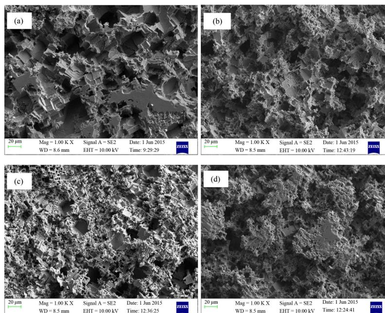
**Figure 8.** The SEM micrographs showing the pores for different concentrations: (a) undiluted acid; (b) 1:1, acid to ethanol by volume; (c) 1:2, acid to ethanol by volume and (d) 1:3, acid to ethanol by volume.
