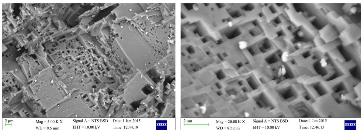
**Figure 9.** SEM micrograph showing magnified minipores within a bigger pore.
