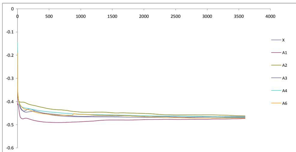
**Figure 3.** OCP measurement for 2205 DSS composites in simulated mine water
