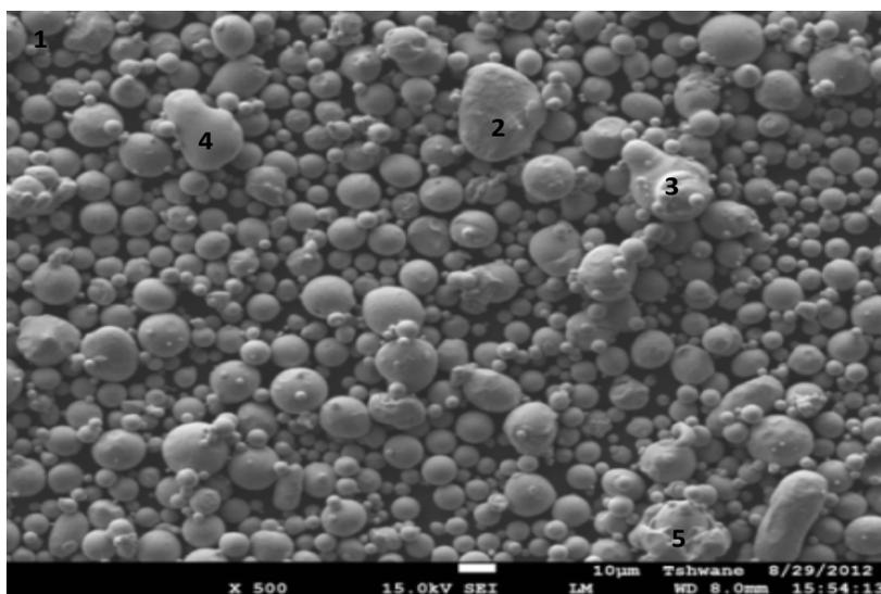
**Figure 1.** SEM image of as-received 2205 DSS powder
