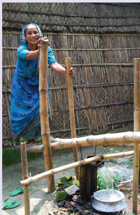
Figure 2.8 – Using an IDE treadle pump this Bangladeshi woman can now support her family and run a small shop
