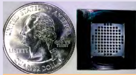
Figure 9.31 – A carbon-nanotube membrane (quarter coin shown for scale) 68
