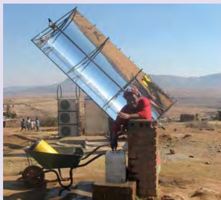
Figure 7.22 – A woman collects water next to a prototype CST system installed by STG International, in Ha Teboho, Lesotho, which generates hot water from a second tap
